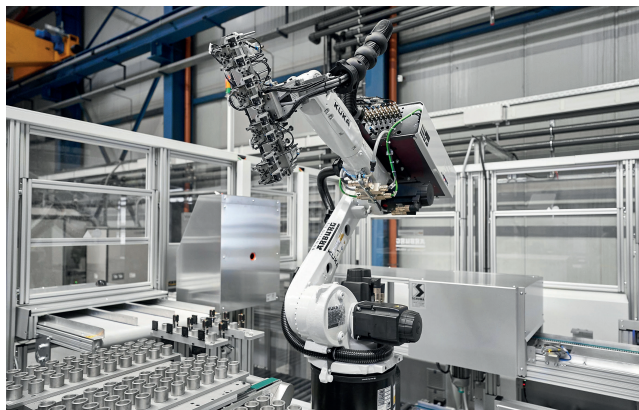
Fig. 2. A six-axis robot feeds the molded parts to the camera inspection (rear area) and sorting and deposits the good parts (front area) © Arburg
